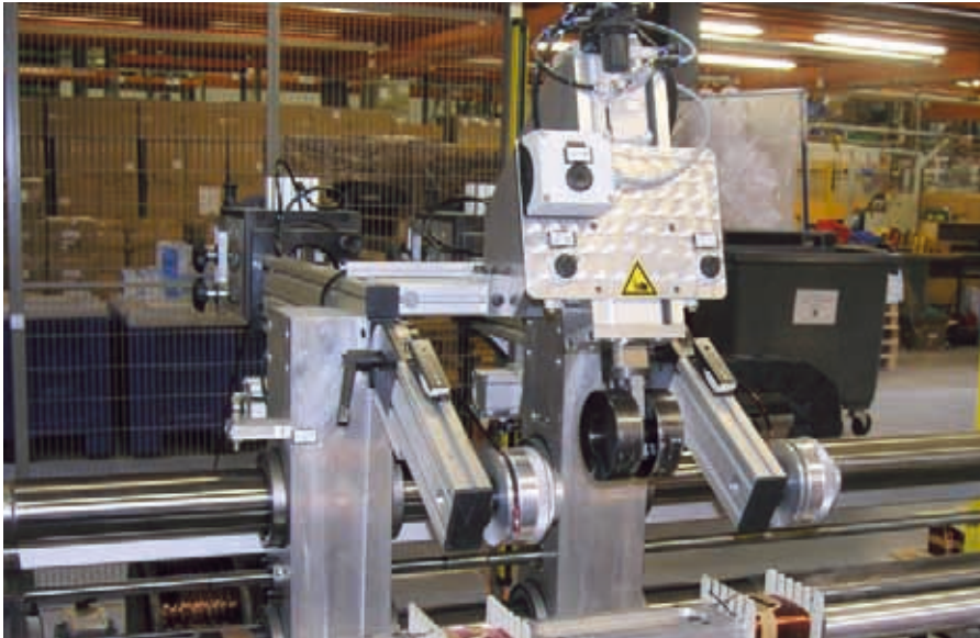
GYS manufactures its transformers and designed a machine to wind copper sheets for a transformer delivering more than 12.000 amps.
