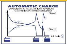
• Fully recharges lead-acid batteries between 40 - 350 Ah (W2 charge curve)
