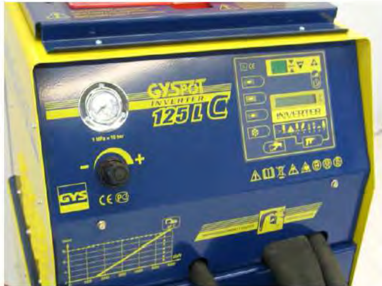
Operating controls and weld tester on the Gys welding machine
