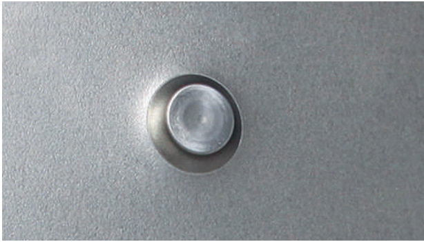
RESULT OF THE INSTALLATION OF SELF-PIERCING RIVET
