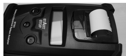
C. Place a small length of paper from the compartment and press the transparent cover to close.
