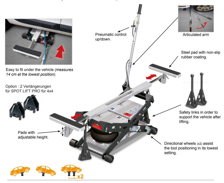
The SPOT LIFT Pro improves productivity by enabling the user to work in a more comfortable position.
