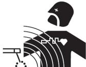
The electric current flowing through any conductor causes electrical and magnetic fields (EMF). The welding current generates an EMF around the welding circuit and the welding equipment.
