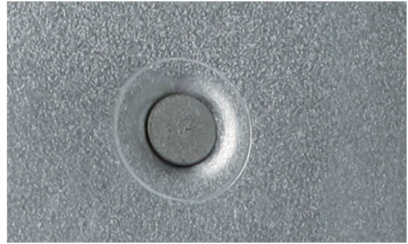
THE OUTCOME OF INSTALLING SELF-PIERCING RIVETS
