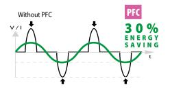
PFC technology eliminates power surges and regulates the power supply current. PFC accepts power supply voltage between 185V and 265V, the use of extension leads and use on power generators. It also helps to provide better arc stability during the welding phase for consistent welding beads.
